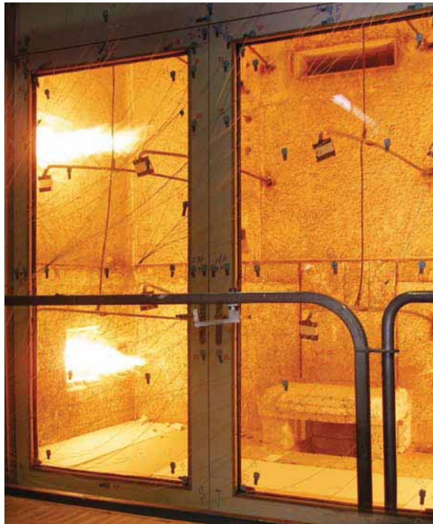
Testing of fire behaviour in accordance with DIN EN 1634-1.
