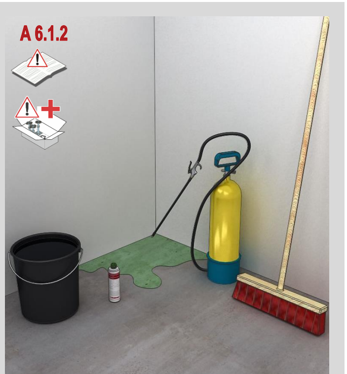
Picture 5 Application of the subfloor sealant
