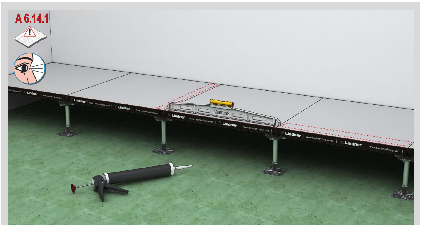
Picture 22 Control of the first row of panels
