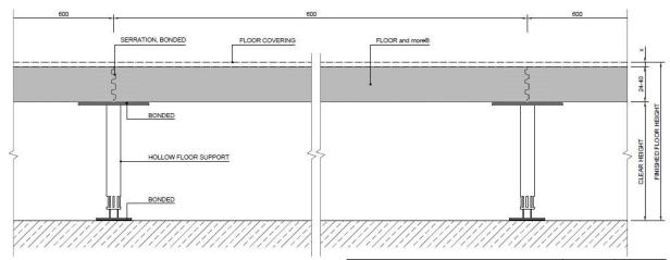
The hollow floor system is in essence formed using hollow floor panels and a substructure.
